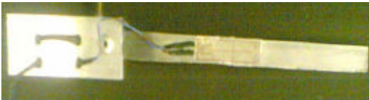
Figure2. Strain gauges use for eccentricity Strain gauges use for side wobbles
